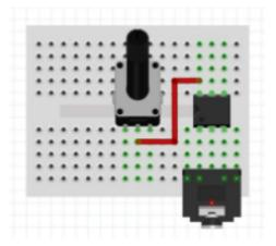
5 Connect your red laser (here represented by the red LED) to the breadboard. Ensure that the ground (black) wire is connected to the upper portion of the breadboard on the leftmost side, and the positive (red) wire is connected to the lower portion of the breadboard.
