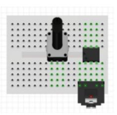
4 Connect the upper left pin of the transformer to the center (wiper) pin of the potentiometer.
