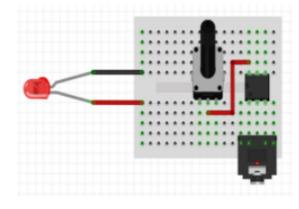
6 Connect the leftmost pin on the potentiometer to the positive (red) wire of the laser.
