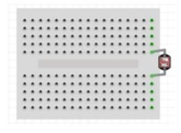
2 Plug the speaker in on the opposite side of the board, bridging the gap between the two sides of the breadboard. The positive (red) wire should be on the bottom half of the breadboard.
