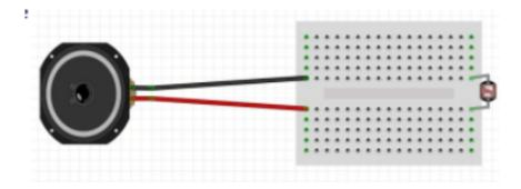
3 Connect the output of the photoresistor (bottom leg) to the input (red wire) of the speaker. Remember, anything in the same column on the breadboard as your wire will be electrically connected!
