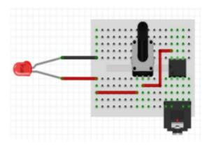
7 Place your 3 AA batteries in the holder above the breadboard. We will soon power the circuit.
